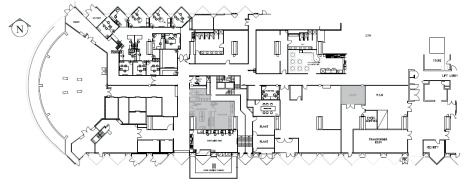
Plan E—The shaded areas are the Administration Area, Count Facilities Area and Secure Storage Area on the lower ground floor level of the casino.
