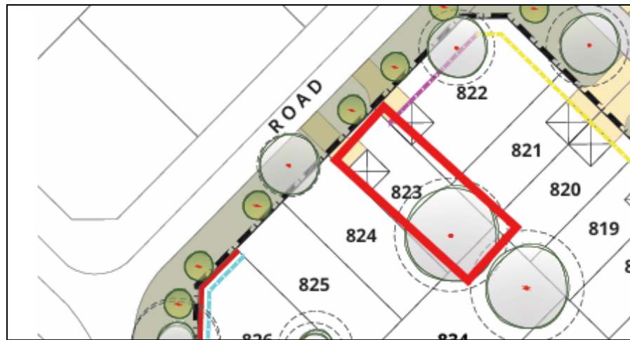
Figure 6 - Tree Protection Zone which overlaps adjoining properties
