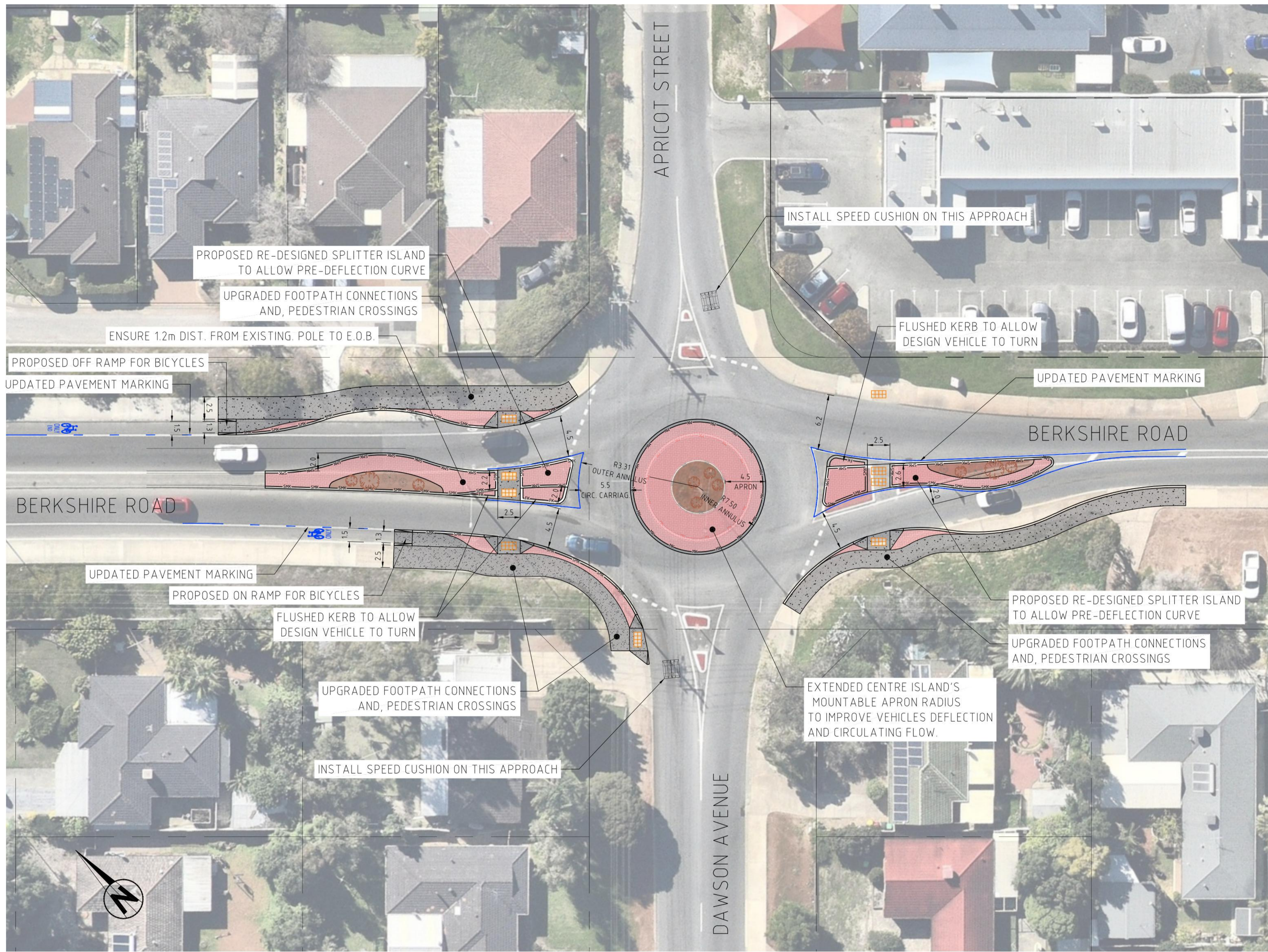
ROUNDBOUT UPGRADES - CONCEPT PLAN SCALE 1:250
