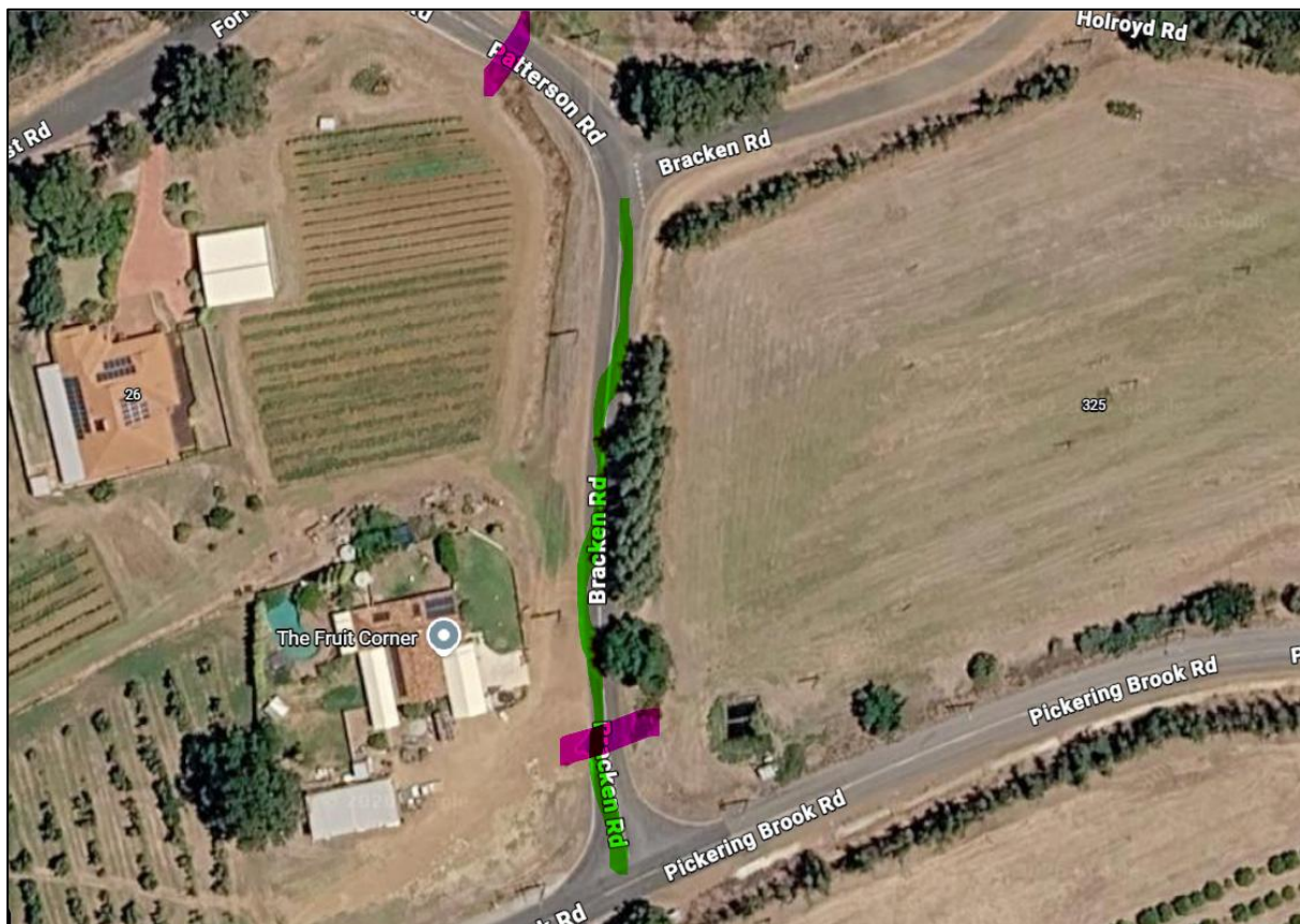
Figure 9.1: This road section is signposted Bracken Road (green). Note culverts restricting road width (magenta).
