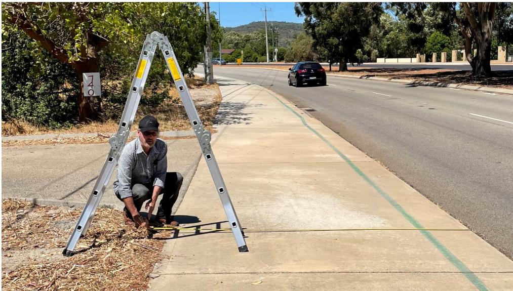
**Photo 4 – Setting up “Height of Eye” observation position for car (1.1m).**
