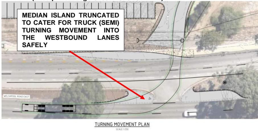
Refer to **Figure 11** below for an overlay showing the potential median refuge situation for a car and trailer combination. A car would certainly have sufficient space to be accommodated, a car and trailer would most likely be accommodated (depending on size of the trailer) but the semi-trailer would not be able to be accommodated.
