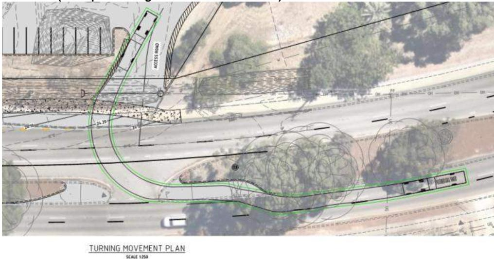
The alternate longer slip lane arrangement has now also been provided for council engineer's consideration and an excerpt is shown in **Figure 8** below (refer also to Drg **PC16017-CI-SK8-REV D** in **Appendix B**) but this will require the removal of existing trees located in the median.
