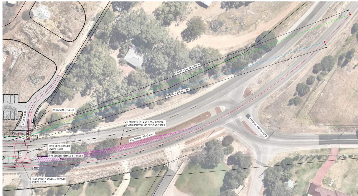
**(SISD) SAFE INTERSECTION STOPPING DISTANCE PLAN 2**
