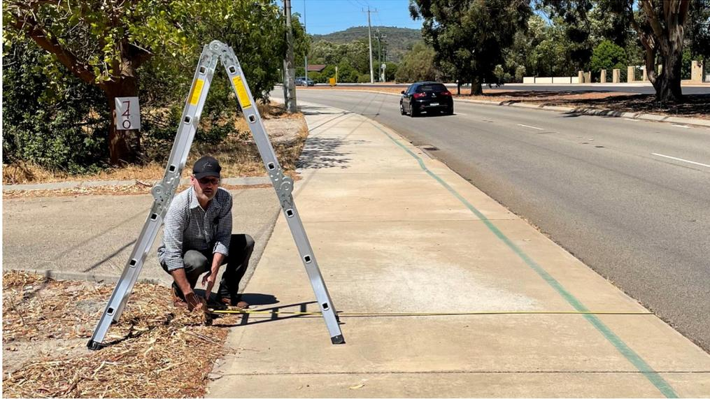
**Photo 4 – Setting up “Height of Eye” observation position for car (1.1m).**
