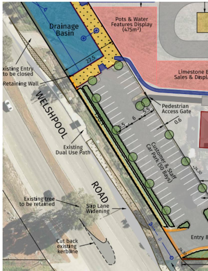
32. The deceleration lane design proposed for vehicles entering the site from the west has a lane distance of 97m. Austroads Guidelines require a lane distance of 125m in order to accommodate a 'comfortable' deceleration speed. The RSA audit has identified this deficiency. The MRWA commentary has noted this deficiency. The distances are calculated on the basis of the posted speed limit plus 10 km/h which is the manner in how they are assessed.
