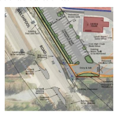
31. Turning Movement a) (from the west into driveway) is proposed to be facilitated by a deceleration 'slip' lane which also incorporates the existing embayed bus bay. This is shown in the following diagram:
