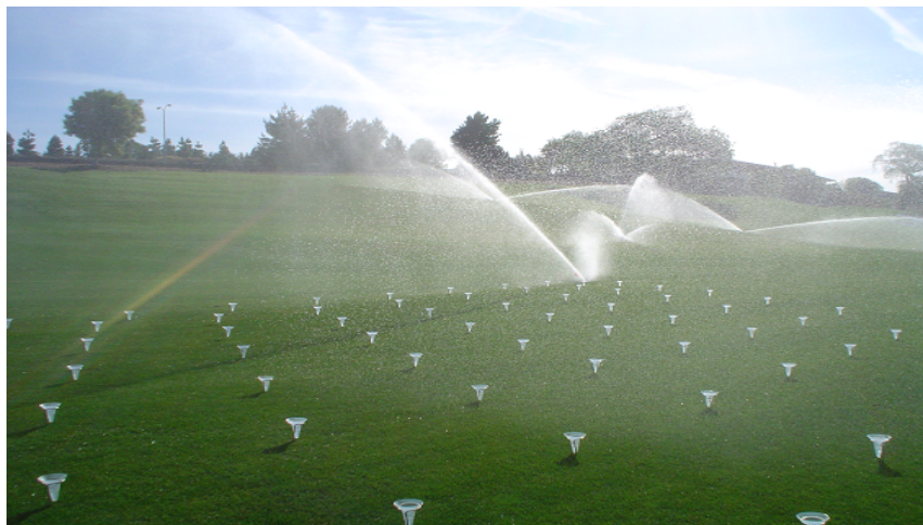
Catch cup test method
