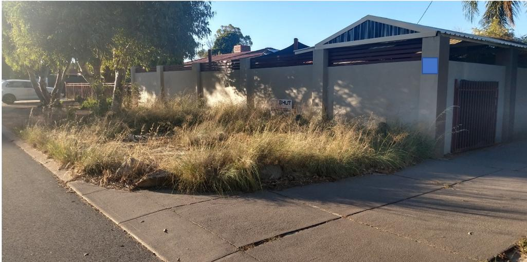
This picture shows that the verge has been covered with gravel and has soil piled up. This treatment is dangerous to mow, with projectiles from mower blades common. Mowing equipment is also often damaged, expensive to repair and not available to use whilst being repaired.
