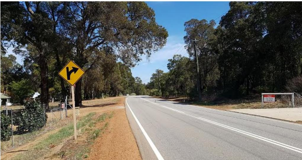
**Photo 41:** The warning sign does not fully identify the connections or potential movements.
