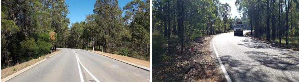
**Photos 3 & 3a:** The bend south of Pickering Brook Road is too sharp for the posted 70 km/h speed limit
