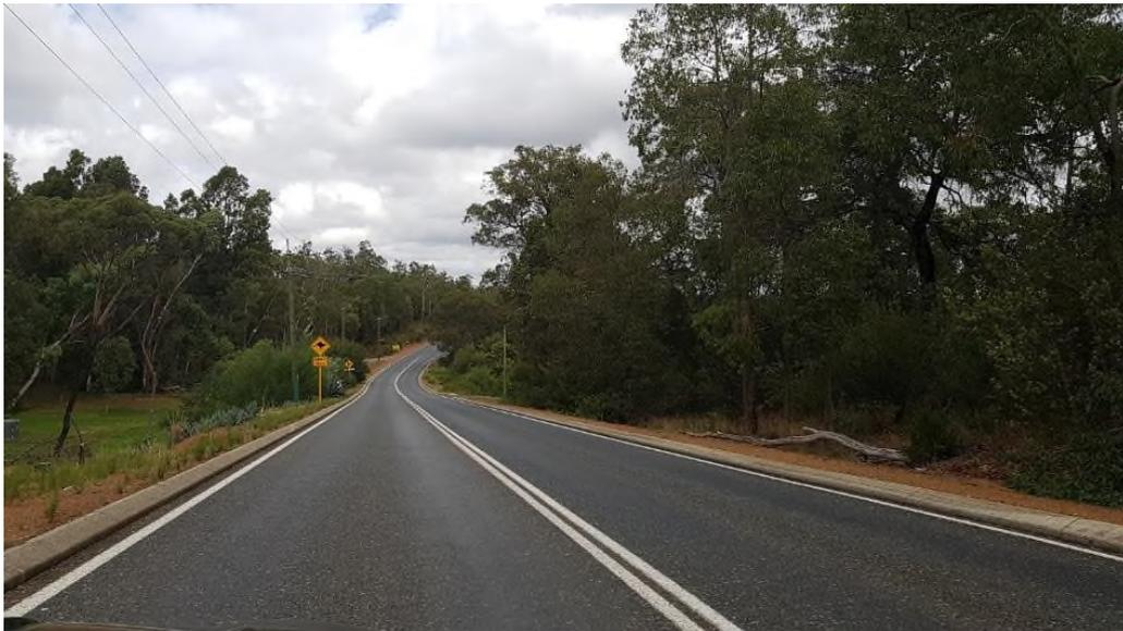
**Photo 2: Typical combined horizontal and vertical curves within this section of Canning Road.**
