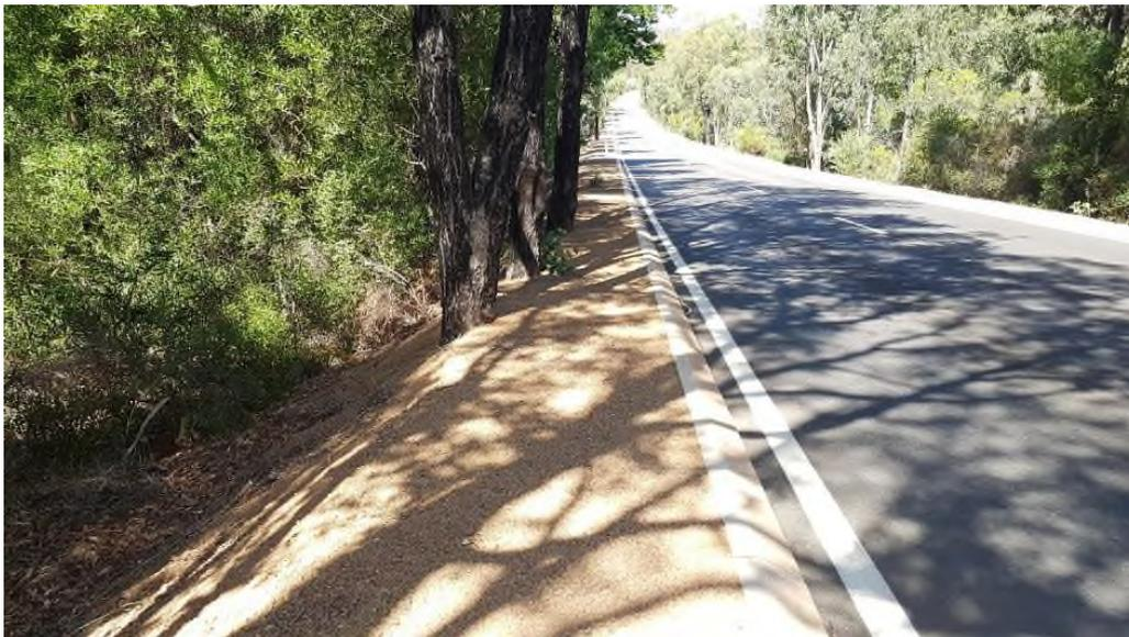
Photo 54: Trees near the road with significant drop off.
