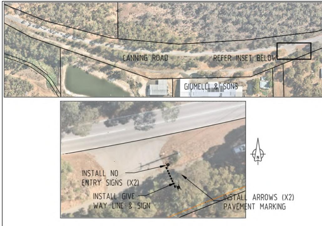
**Figure 4.2: Temporary safety improvements at eastern access to Guimelli & Sons**
