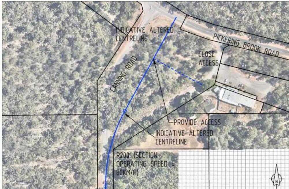
Figure 4.3: Conceptual realignment of Canning Road at Pickering Brook Road
