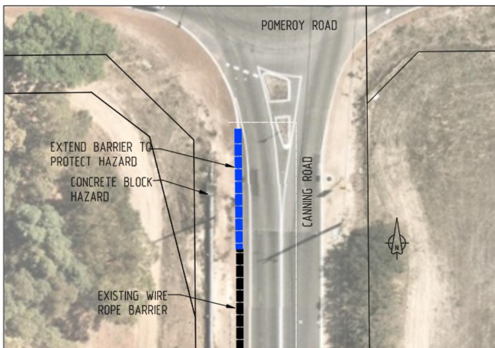
**Figure 4.1: Recommendation to extend safety barrier north to protect existing hazard**
