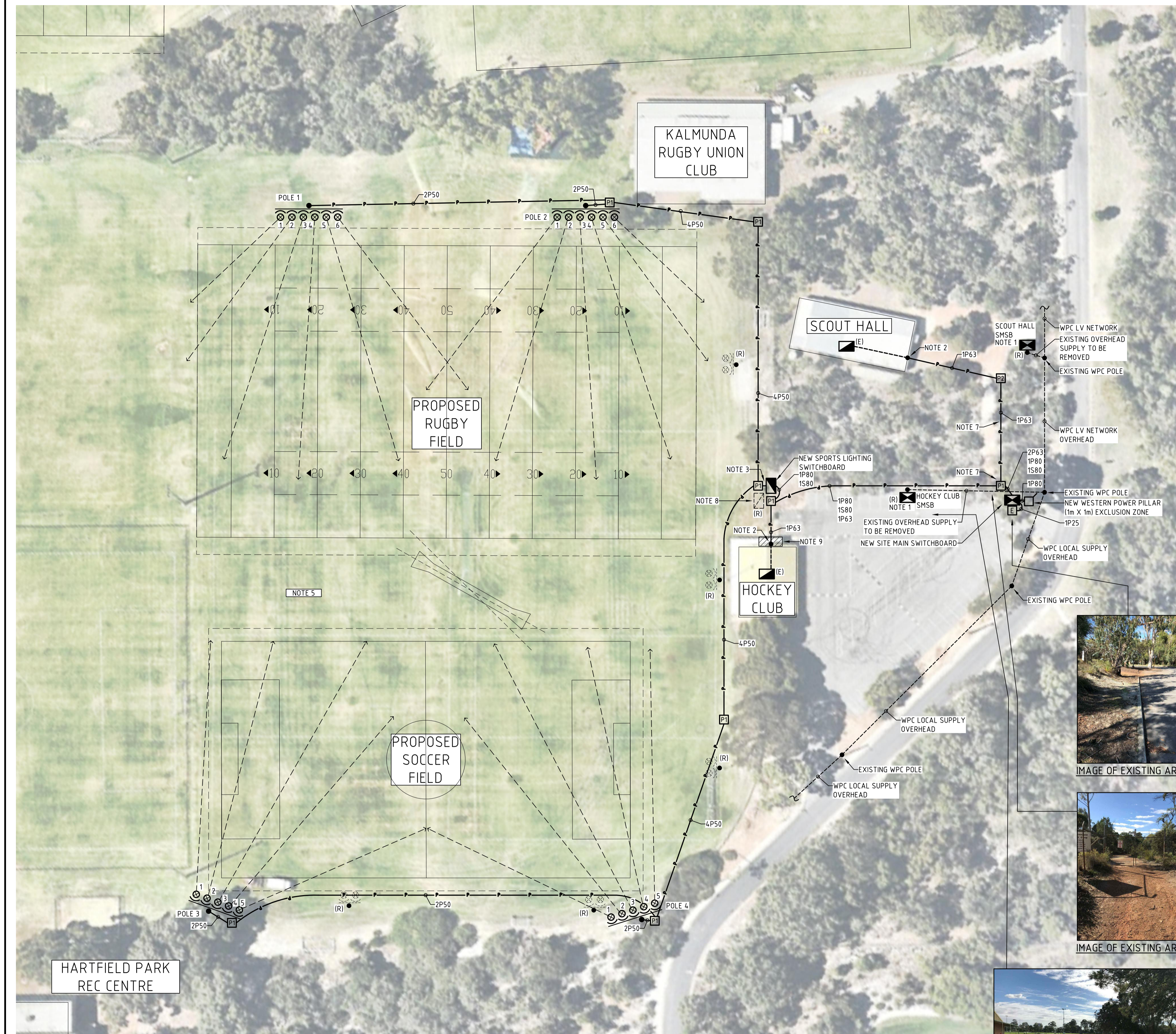
SITE PLAN - SPORTS LIGHTING LAYOUT SCALE 1:500 @ A1
